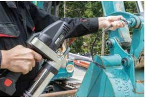
One-touch locking for confined spaces. Designed to access recessed grease fittings in tight areas -no slipping, no mess. Just grease firmly.
