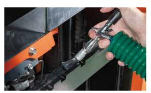
Efficient Coverage for Heavy-Duty Equipment Specialized brush ensures smooth, uniform grease distribution across -ideal for use on construction, farming and industrial machinery.
