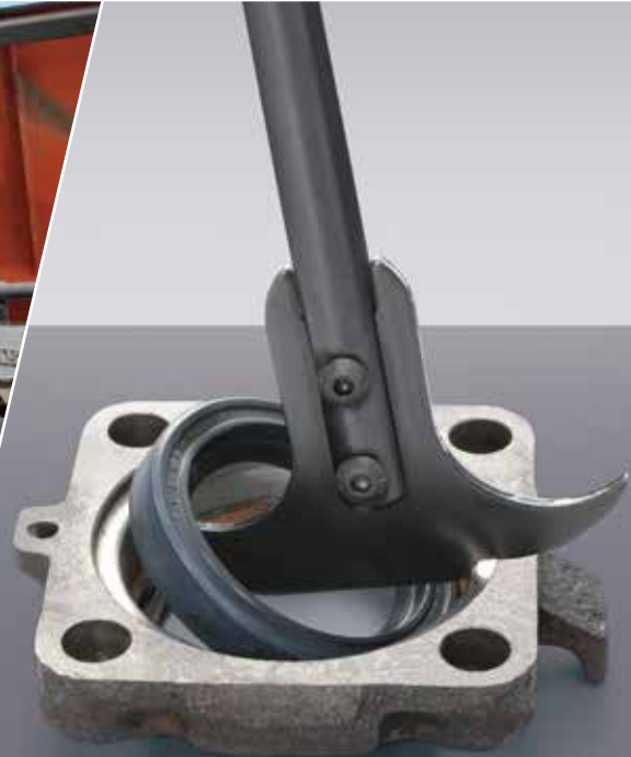
Oil seal removal on agricultural machinery
