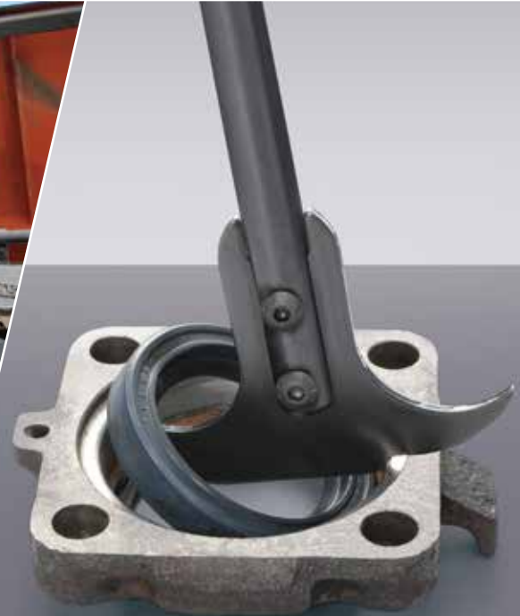
Oil seal removal on agricultural machinery
