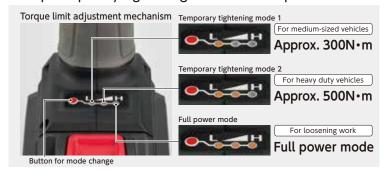
Press the switch mode button to switch between 3 modes. Quick and efficient tightening by using the pre-tightening mode that prevents over-tightening of wheel nuts.
