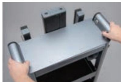
Install lifting switches in handle section and require both hands to operate at the same time to avoid wrong and unexpected running.
