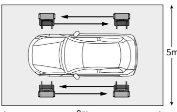
Smooth move even in the limited space. Improve efficiency of the tire rotation work with rotation cart (AWR101).
