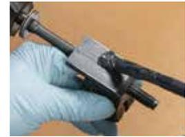
③ Lubrication of screw parts
