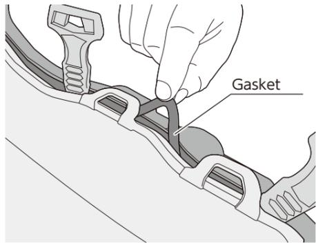
5. Pull the gasket out through the gap where you inserted the headlamp wedge.
