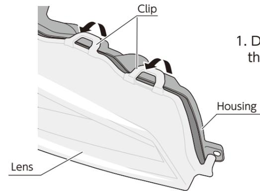
1. Decide where to insert the plier and release the clip connecting the headlamp lens to the housing near that point.
