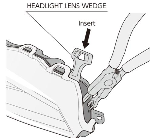
3. Insert headlamp wedge into the gap opened by the removal plier. You can remove the plier as long as you can insert it firmly.
