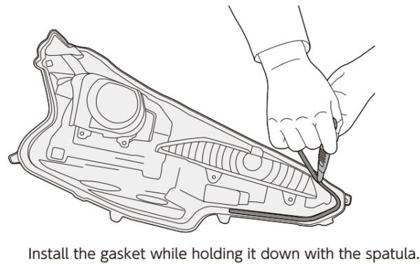
2. Install the gasket around the circumference, and complete by aligning the housing and the lens.
