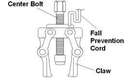
• Pitman arm may spring off with big sound or the puller may fall off the moment pitman arm is pulled out. Be sure to tie the fall off prevention cord to rigid section of the car.
